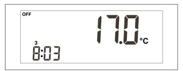
Entering this mode gives access to the configuration values that could have been changed temporarily, the set points and fan status.
