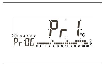
If the communication profiles are not empty, which means they are not on 24-hour stand-by, or a profile above the first six (three predefined and three user-programmable) has been selected by means of communication with the PC, profiles P7 to P12 can be selected. Should this not be the case, these profiles can neither be selected nor are displayed on screen.
