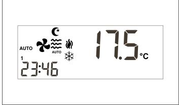
A demand is generated when the room temperature is above the cooling set point or below the heating set point. In automatic mode, room temperature is kept at a value between these two programmed set points.
