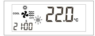
A demand is generated when the room temperature is above the programmed set point. Set point is understood as the temperature we want in the room. How to program and change set points will be described further below.
