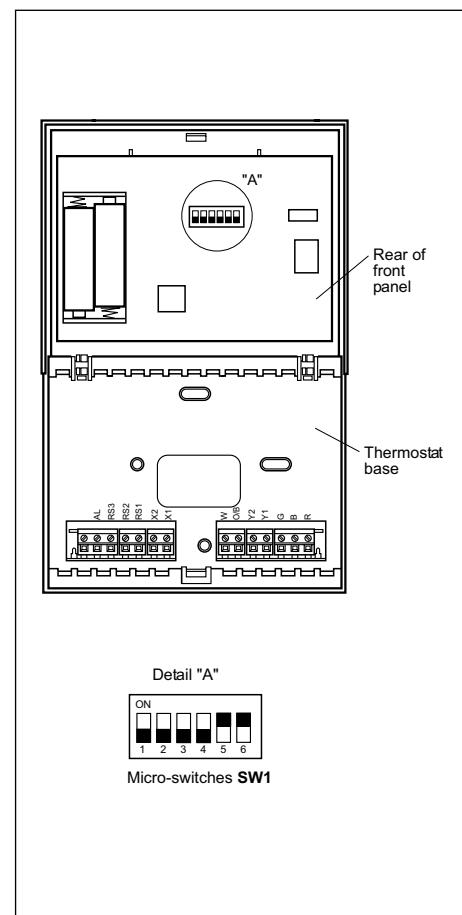
Micro-switches SW1 allow the configuration of the following parameters:
