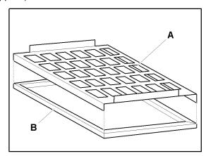
Fit the filters **-A-** next to the shutter grille in the top and bottom economiser rain protection sections.
