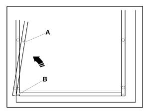
Re-position the left-hand side panel **-A-** vertically and line up the holes in it with those in the vertical support (hidden by the rubber strip).
