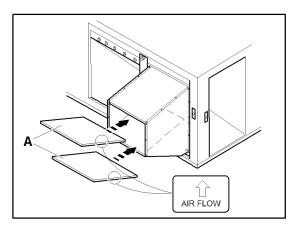
Fit and secure the equipment access panels.
