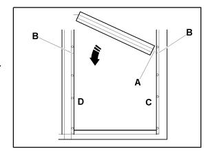
Push the left-hand side panel -A- to the left and raise the central panel in the zone -B- until the rear tab - C- fits into the groove in the left-hand side panel.
