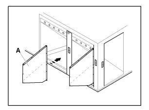
Tilt the left-hand side panel **-A-** to the right and fit so that the tab **-B-** on the lower filter support can be inserted into the groove at the bottom.
