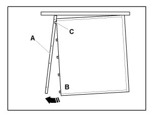
Bend the two tabs on the lower filter support upwards and all the others on the central panel downwards.
