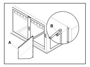
Tilt the lower filter support **-A-** so that the tab fits into the groove on the right-hand side panel. Then lower the support so that it rests on the equipment frame.
